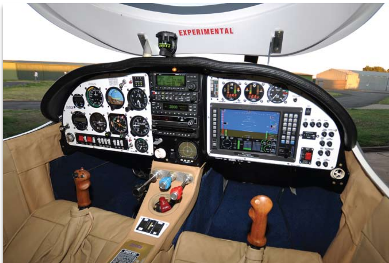
Four inches of additional width has been built into the Legacy. However, the cabin is not a place for big pilots and passengers.
